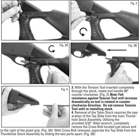
5. Separate Top Slide from shotgun. The Top Slide is attached to the shotgun with a preinstalled bolt and lock washer. To loosen bolt, insert a ¼" or 3/16" Allen Wrench (T-Handle Wrench Recommended) into the opening located on the bottom of the slide. Turn wrench counter clockwise until Aluminum Slide is free from shotgun. (Fig. 4) Stock removal complete. Reinstall cross bolt; leave tension tool inserted into stock when storing.
