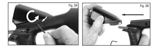
**4. NOTE:** Remove rubber o-ring from stock bolt. Remove o-ring by inserting allen wrench into hole located in the back of the Top Slide. Turn wrench counter clockwise while applying pressure to the bolt with finger. Turn wrench until rubber o-ring is removed. **NOTE:** For all stocks, the rubber o-ring is for packaging use only. If a loose o-ring is found in the stock packaging, disregard and dispose of it.
