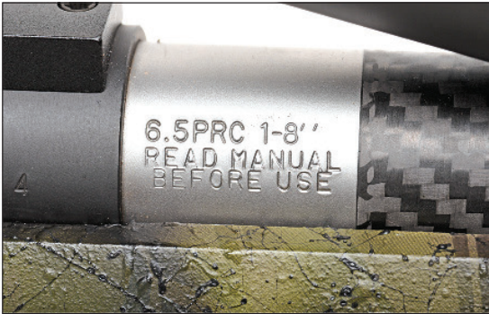
Barrel twist is 1 turn in 8 inches.
