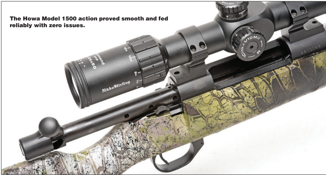
The bolt handle is long enough to provide plenty of leverage and a 3-position safety is standard.
