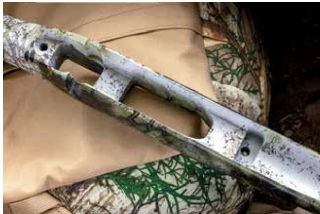
The stock has sling swivels fore and aft, and the internal recesses correspond to the action's integral recoil lug and flat bottom.
