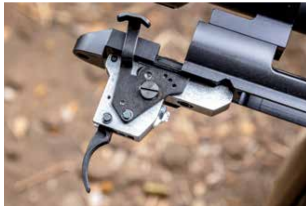
The two-stage HACT trigger from Howa came set at just more than 4 pounds. It was user-adjustable to just less than 3 pounds.
