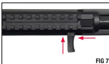
To keep the bolt in an open position without the magazine, pull the bolt to its most rearward position and press the bolt lever towards the receiver (in the direction shown by the engraved arrow) (fig. 7).
