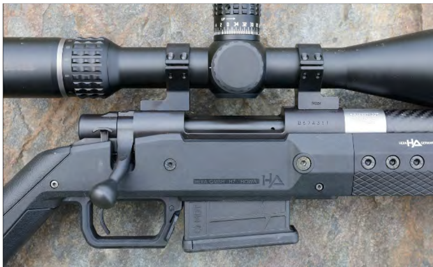
The 1500 action is at the heart of the Hera. It feeds from AICS magazines, but an aftermarket conversion kit allows you to change it to a hinged floorplate.
