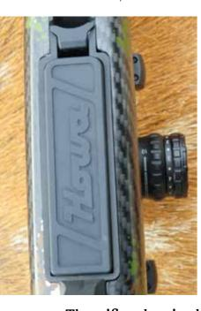
action and three-position safety on the right are stamped steel so lacked a bit of finesse. The safety blocks the trigger and allows safe cycling of the bolt in the middle position another useful feature.
