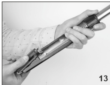
13. Pull back and remove the mechanism
