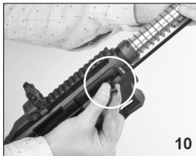
10. Remove the charging handle by pulling it
