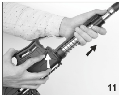
11. Turn the bolt catch lever.
