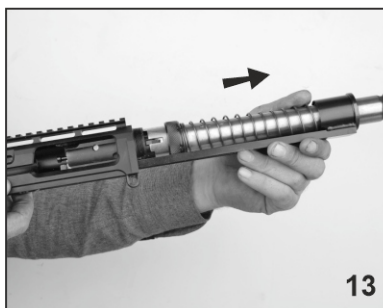
13. Pull out the assembly in arrow direction
