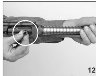
12. Remove the charging handle by pulling it
