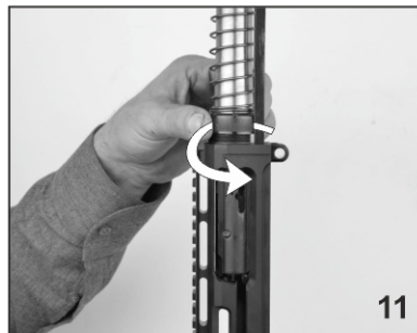
11. Turn the barrel nut in the direction of the arrow.
