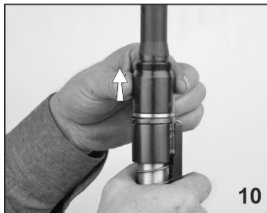
10. Remove the piston by pulling in arrow direction.
