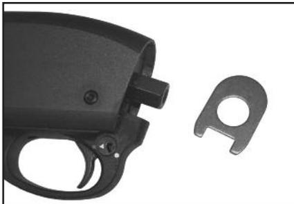
**NOTE:** Remington owner, after installation, there should be no gap between the stock and receiver. If there is a consistent 1/8" gap between the stock and receiver verify that the metal spacer has been removed. The spacer is not needed for installation of the Talon Stock.
